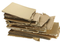
Corrugated Cardboard (Wavy center layer)
