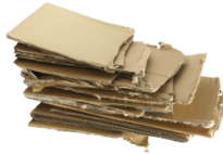
Corrugated Cardboard (Wavy center layer)
